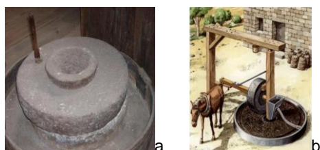
Fig. 2 Roman grindstone a) manual drive; b) animal drive
