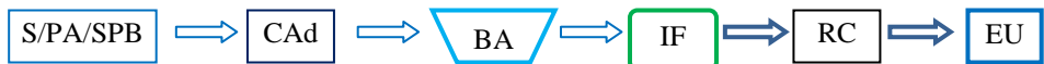
Fig. 1 Groundwater source irrigation system design scheme: S / PA / SPB - water source / pump / pumping station; CAAd - conduit; BA - storage basin; IF - frontal installation; RC - pipeline network; EU - watering equipment
